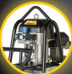
**Air motor** Easy to handle, with soft-start function and full pressure steering for excellent reliability.
